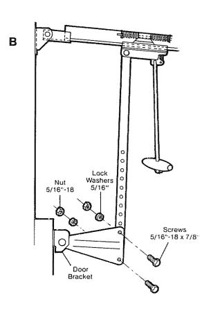
Bring the door arm sections together. Find a pair of holes that line up and join sections as shown (B).
